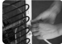
connect the PE tube to input connection
